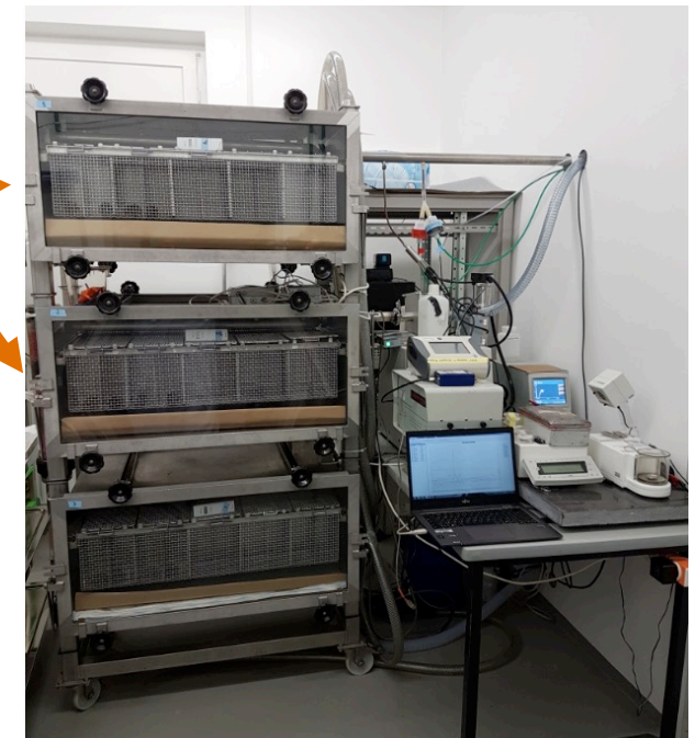
Whole body single housing inhalation exposure units
